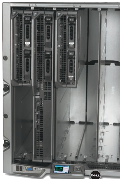
Figure 2. Full-height and half-height blade servers side by side in the Dell PowerEdge M1000e
