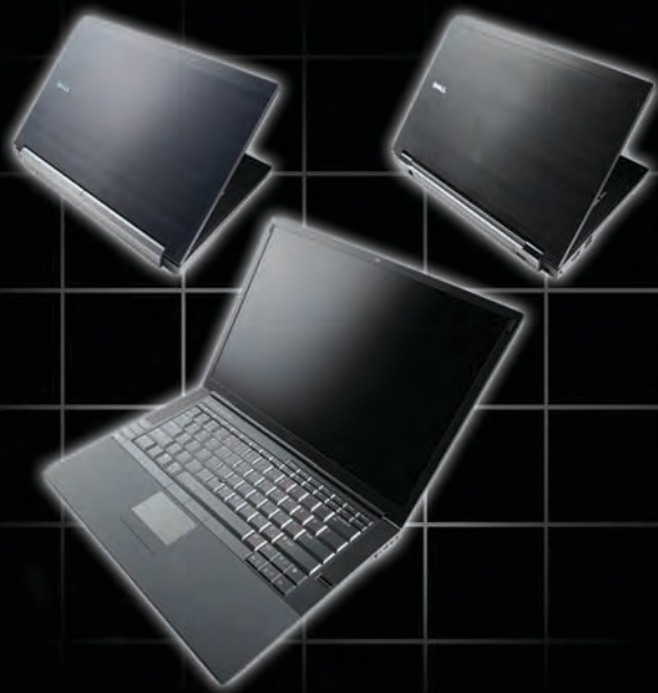
Step 6: Full-scale hard models are built to guide selection of the final designs, clearing the way for the Dell engineering teams to finalize the internal components.
