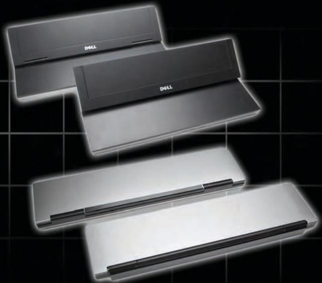
Step 5: Various hard models of subcomponents are crafted to demonstrate key design attributes. In this case, hinge models show the design progression from previous-generation Latitude D-Family laptops (background) to the new Latitude E-Family laptops (foreground).
