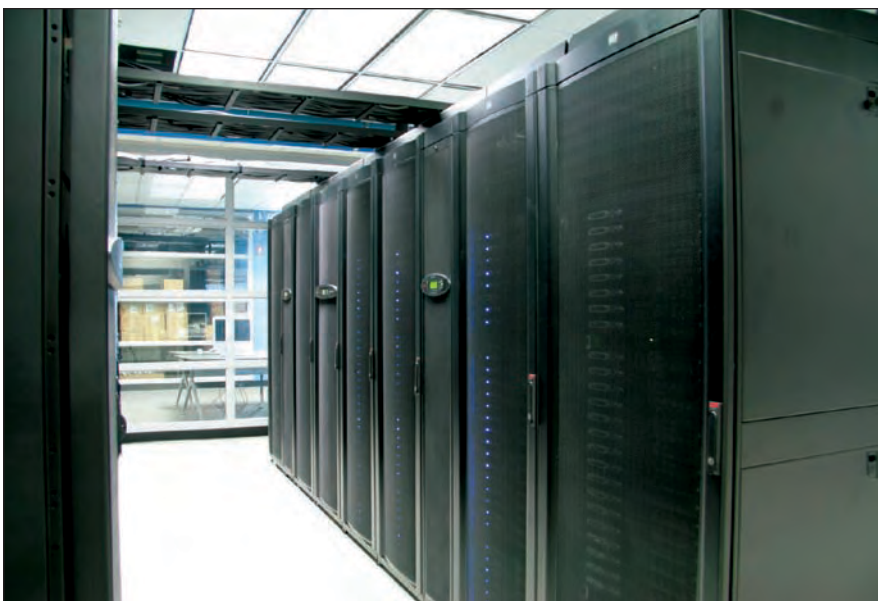
Figure 2. The HCC cluster is based on 1,150 Dell PowerEdge SC1435 server nodes and a PowerEdge 6950 master node
