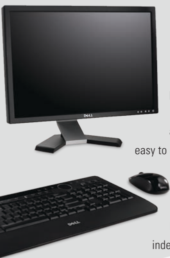
Supporting flexible peripherals: Dell E-Flat Panel Stand integrated with Dell E-Port docking station
