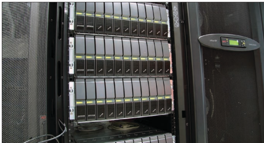
Figure 3. Panasas storage provides the HCC cluster with over 150 TB of space over Fibre Channel links
