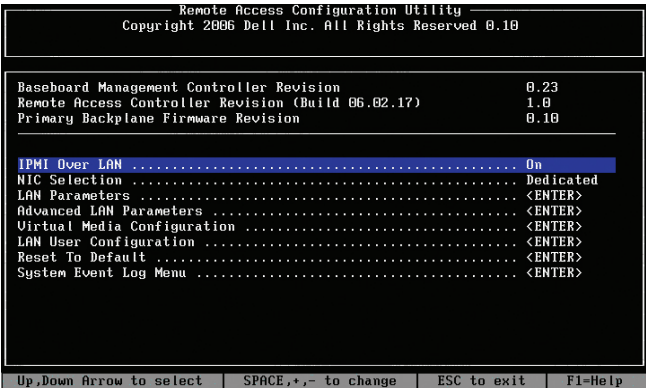
Figure 1. NIC Selection field in the BMC BIOS binary option ROM
