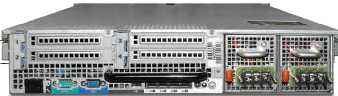
Hot-swappable hard drives and redundant power supplies help maximize E-2710 reliability and uptime
