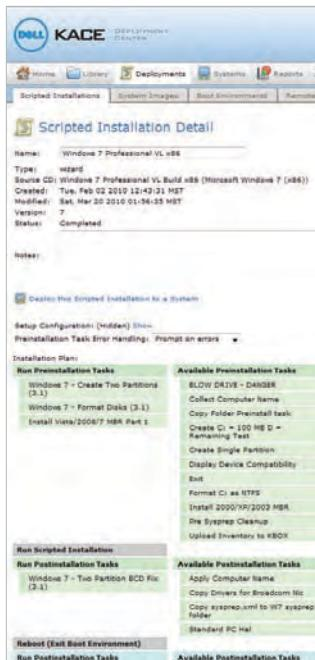
**Figure 1.** Scripted installation details in the Dell KACE management interface
