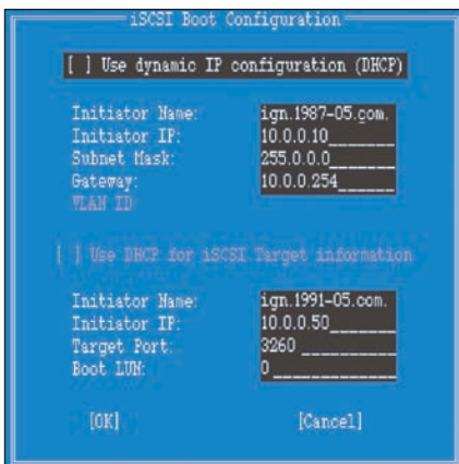
Figure 2. Intel iSCSI Boot Configuration menu using centralized DHCP configuration
