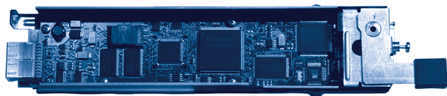
Figure 1. Avocent Analog KVM switch module for the Dell PowerEdge 1855 blade server
