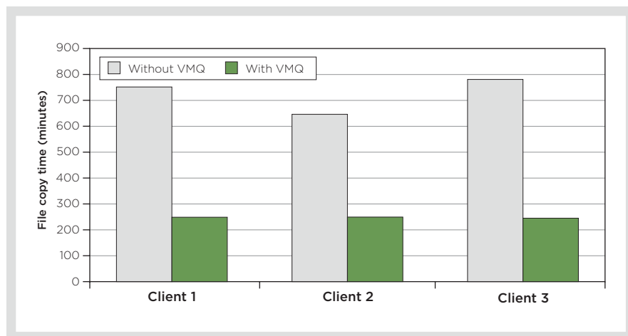
Figure 4. File copy times with and without the VMQ feature enabled
