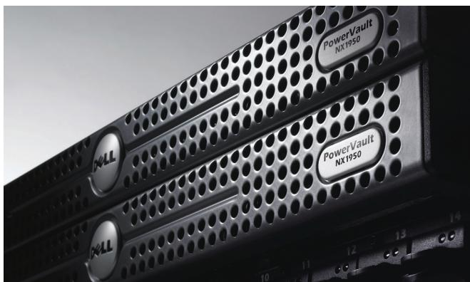
The Dell PowerVault NX1950 is a unified network storage solution that simultaneously stores both file and application data and supports a wide range of operating environments and communication protocols, including Internet SCSI (iSCSI). See page 43.
